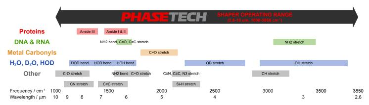
The QuickShape operates at wavelengths covering the most-studied vibrations of proteins, DNA & RNA, metal carbonyls and water. Other wavelength ranges are also available by request.
